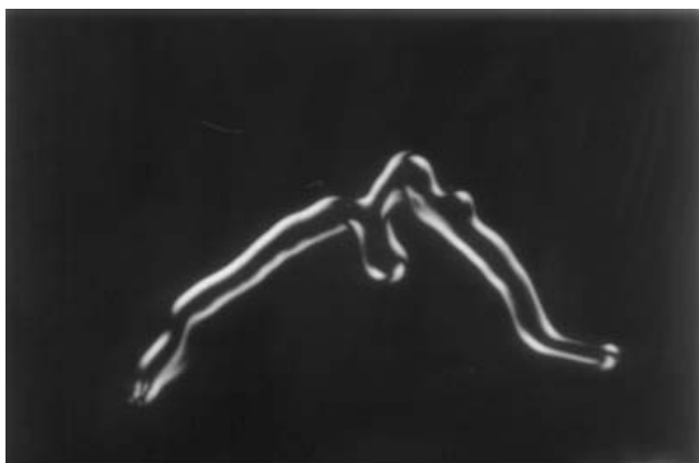
Figure 1. Photomicrograph of a filament growing on cooling the isotropic phase of compound 22 at 153.8^{\circ}\text{C} ; magnification \times 200 .
